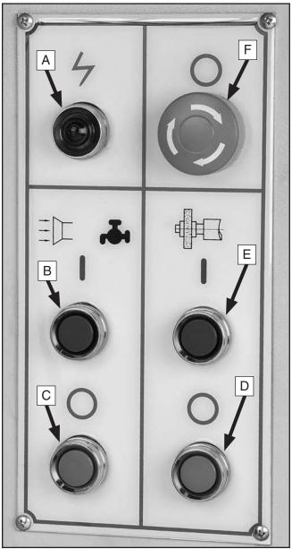
Figure 2. Grinding wheel and coolant controls.
